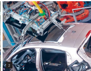
2 GVMAX vacuum pumps and VPYR ball joint suction cups for handling of glazed elements
